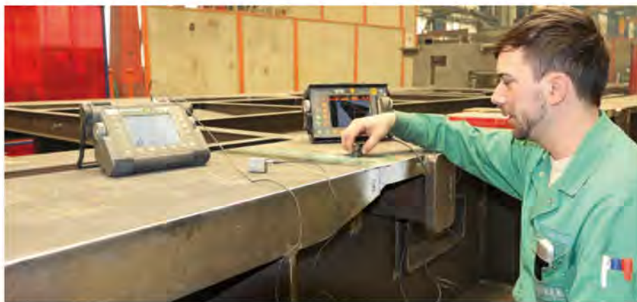
Non-destructive testing (ultrasonic) of a full-depth weld seam
